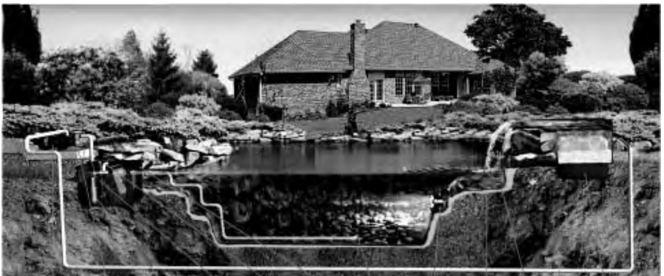
Out-Of-Pond Pump Leaf Basket Oil-less Submersible Pump Pump Cut-Off Switch Discharge Kit Skimmer Bottom Drain Kit Low-Voltage Submersible Light Sand Base EPDM Liner PVC Pipe Biological Waterfall Filter
